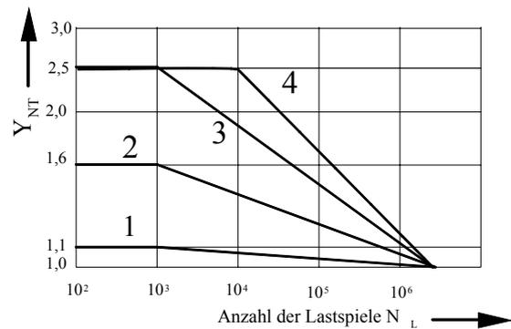
Fig. 11: Life curve for gear wheel face
