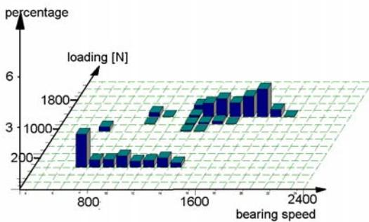
Fig. 5: loading speed characteristic of a bearing
