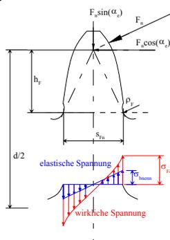
Fig. 9: Forces and stresses on a gear wheel
