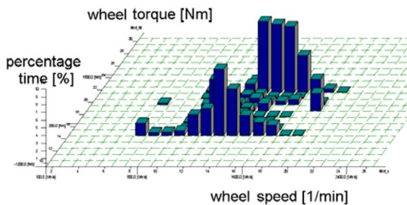
Fig. 4: torque speed characteristic of a gear wheel
