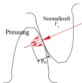
Fig. 10: Forces in the face of a tooth
