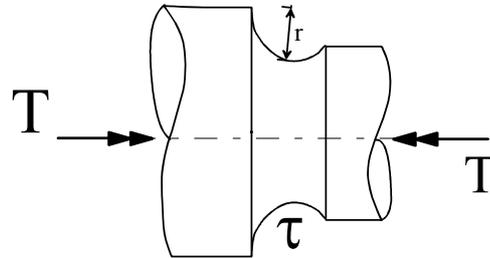
Fig. 6: critical area of an axle under torque loading
