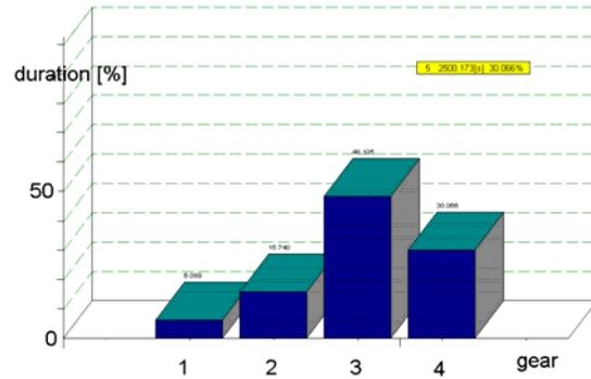
Fig. 1: Percentage of time for gear speeds of a city bus in a city of Germany
