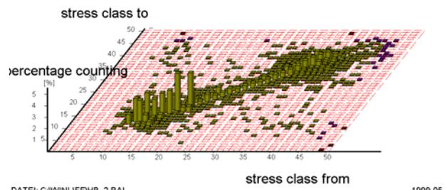
Fig. 7: typical result of a rainflow counting of an input torque
