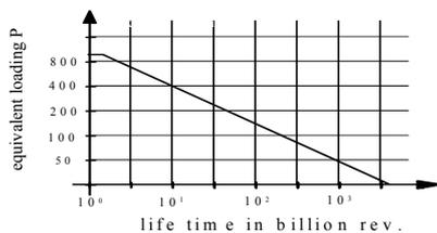
Fig. 14: characteristic of life curve for ball bearing
