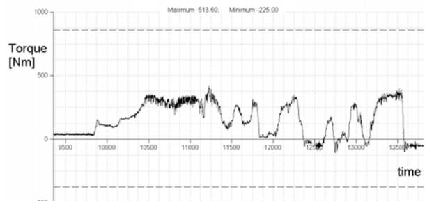
Fig. 3: Time history of the input torque for a fatigue calculation of axles.
