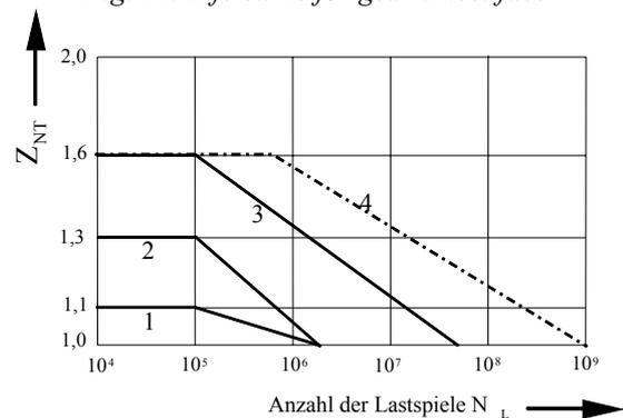
Fig. 12: Life curve for gear wheel base
