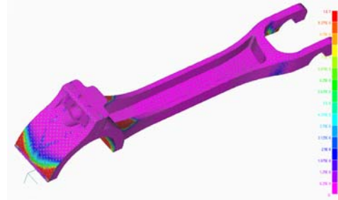
Figure 11: component of a truck suspension, which was used to predict fatigue life
